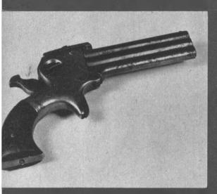
The swing to automatic pistols in the 1860's brought multi-barreled guns like this one into existence. It is a .30-caliber Marston and fires from three barrels.
